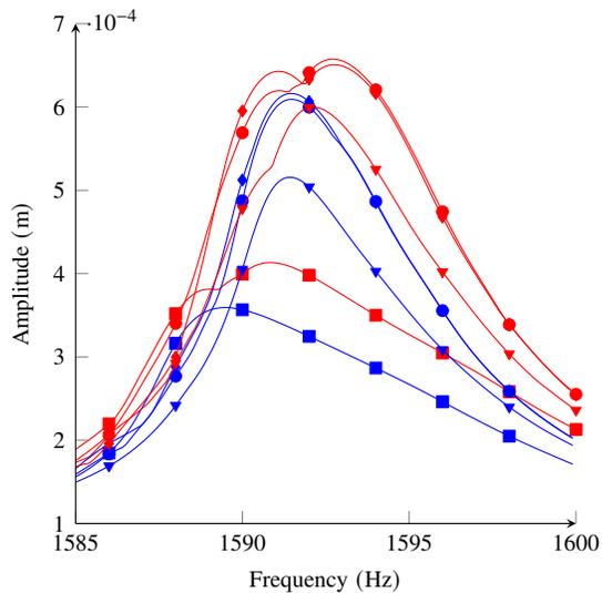
**FIGURE 10: FREQUENCY FORCED RESPONSES FOR THE 1F MODE FOR THE SIX BEST STRUCTURES. (—): WITHOUT RANDOM MISTUNING; (—): WITH RANDOM MISTUNING. THE MARKERS (■), (▼), (●), AND (◆) DENOTE THE (A)<sub>24</sub>, (AB)<sub>12</sub>, (2A2B1A1B)<sub>4</sub> AND MP345 SYSTEMS.**
