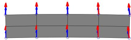
FIGURE 7: ILLUSTRATION OF THE DEFORMED SHAPE OF THE RIGHT UDP BOUNDARY SURFACE FOR THE 1F MODE. DIRECTION AND AMPLITUDE OF THE MAXIMAL DISPLACEMENT FOR: [→] THE  $(A)_{24}$  STRUCTURE, AND [→] THE  $(B)_{24}$  STRUCTURE.
