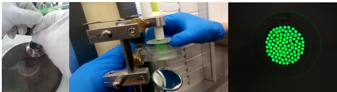
Figure 4: Fiber ends are melted in order to get a flat, smooth surface (left) and are glued inside the cookie (center). A photograph of a ready cookie (right).
