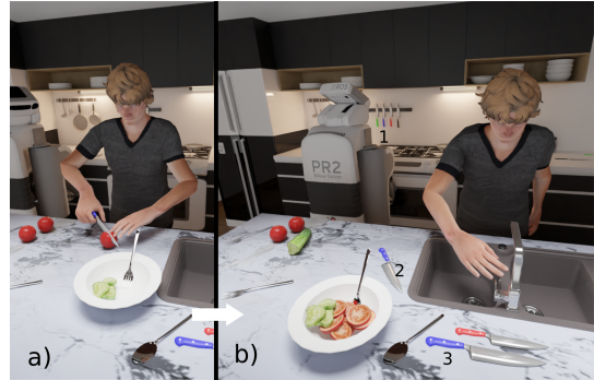
Fig. 1. Referring to knife 2 in the current situation (b) is impossible if the robot is performing an action that does not allow it to see what is in front of the human. Considering a previous step of the human’s task, the robot can refer to the knife through the action to cut a tomato (a).
