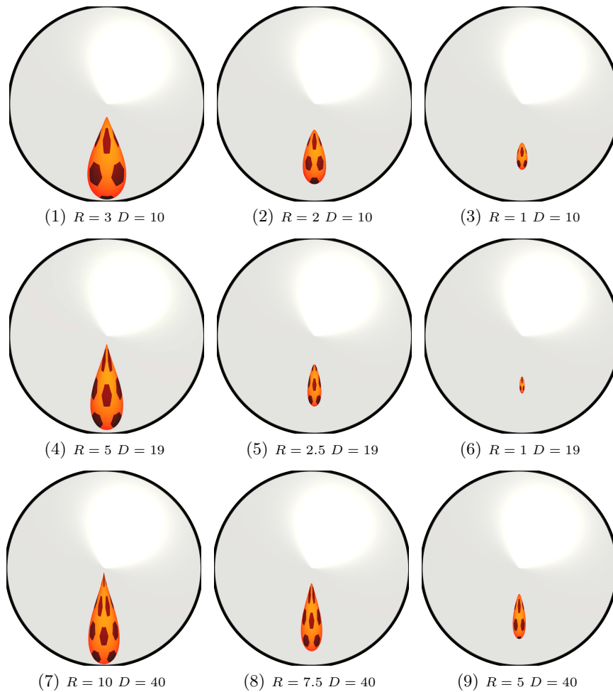
Fig. 4. The set of rendered images used in our experimental activities. The mirror has been modeled as a highly-reflective cone with a semi-aperture of 45^\circ and radius of 5\text{cm} . The cone is placed in front of the (virtual) camera such that the symmetry axis of the mirror and the optical axis coincide; the ball has been modeled as a sphere of radius varying from 1\text{cm} to 10\text{cm} and placed at a distance varying from 10\text{cm} to 40\text{cm} far from the mirror axis.
