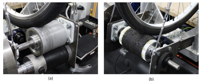
FIGURE 4. Wheel-road surface interaction system (a) before and (b) after the installation of the asphalt specimen.
