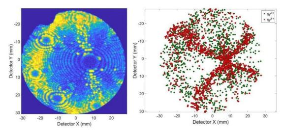
Figure 2: Image formed from field ionised events on the detector (left) and hit positions of the identified W ions on the detector (right) consistent with field desorption maps seen from APT runs of pure W.
