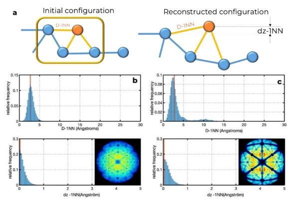
Figure 4: (a) schematic of the initial and reconstructed atomic configurations, and the calculated quantities: the first near-neighbour distance D-1NN and the z-offset dz-1NN. D1NN and dz-1NN for atoms initially on the same plane in the input data in (b) a reconstructed FIM dataset (inset is the multilayer detector map); and (c) the corresponding reconstructed APT simulated data.
