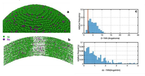
Figure 5: (a) simulation cell with Re segregated to stacking faults in Ni and (b) thin slice though the reconstructed simulated data. (c) D1NN and dz-1NN for Re atoms initially on the same plane in the input data in orange and in the simulated and reconstructed data in blue.
