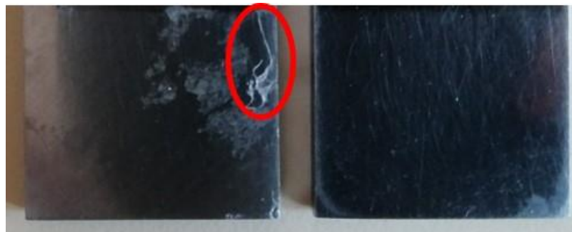
Fig. 5. Images of the two API 5L X65 carbon steel electrodes of surface area 7.5 cm 2 after 97 hours of immersion in 0.5 M NaHCO 3 + 0.2 M NaCl and corrosion products removal (test 5).
