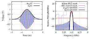
Fig. 1. Up-converted Gaussian pulse truncated at 22% and compliant with the channel 3 frequency mask of the IEEE 802.15.4 standard.
