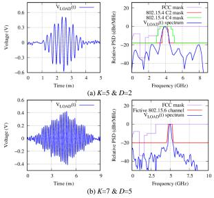
Fig. 9. Example of pulses with the shorter (a) and the longer (b) envelope having a sidelobes rejection higher or equal to 20dB.
