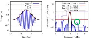
Fig. 3. Example of a pulse with sample & hold Gaussian envelope compliant with the channel 1 of the IEEE 802.15.6 standard (K = 7, D = 2; the highest sidelobes in adjacent channels are circled in green).
