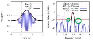
Fig. 2. Example of a pulse with sample & hold Gaussian envelope compliant with the channel 3 of the IEEE 802.15.4 standard (K = 5, D = 3; the highest sidelobes in adjacent channels are circled in green).
