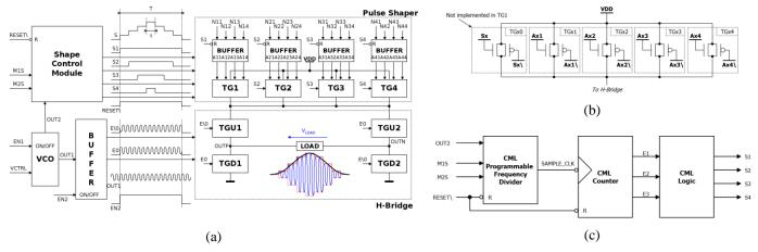
Fig. 4. Architecture of the pulse synthsizer (a), the transmission gates bank (b), the shape control module (c).
