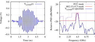
Fig. 7. Pulse for the channel 3 of the IEEE 802.15.4 standard (mandatory).
