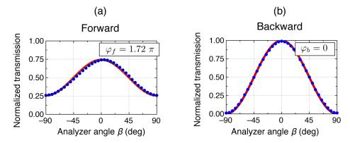
**Fig. 3.** Same as Fig. 2 for the case where the effective wave plate has a general retardation value (close to a  $\lambda/8$ -plate) in forward direction (a) and is a neutral null retarder in backward direction (b). Here  $\lambda = 632.8$  nm and  $\theta_1 = \theta_2 = 77.3$  deg, so that  $\varphi_f = 1.72 \pi$  and  $\varphi_b = 0$ .
