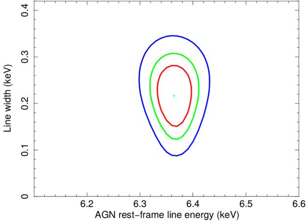
**Fig. 2.** Contour plot of the Fe  $K\alpha$  Gaussian line width (keV) versus its energy (keV), assuming an underlying cutoff power-law continuum over the 3–79 keV energy range (see Sect. 4). The red, green, and blue curves show the confidence levels at 68% ( $\Delta\chi^2 = 2.3$ ), 90% ( $\Delta\chi^2 = 4.61$ ), and 99% ( $\Delta\chi^2 = 9.21$ ), respectively.
