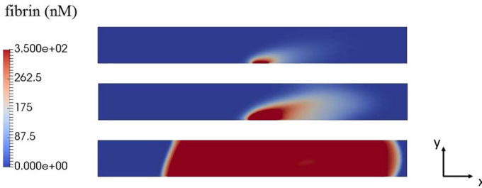
Fig. 8 The concentration of fibrin polymer for a final clot shape for hemophilia (upper figure), healthy (middle figure), and thrombotic (lower figure) subjects. Fibrin clot corresponds to the area with a high concentration of fibrin polymer (red). The corresponding flow velocities are shown in Fig. 7 (Color figure online)
