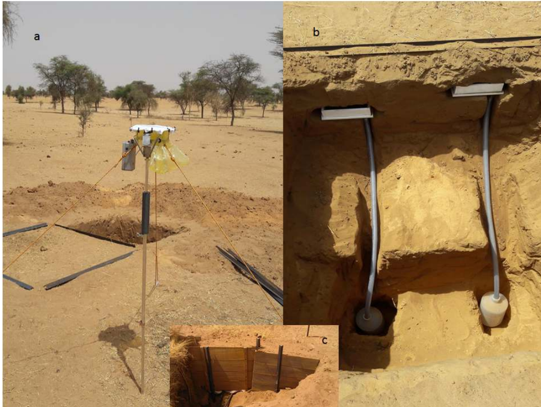
Figure 2: (a) Precipitation collector for rainwater chemistry and (b) lysimeter plates connected to bottles for soil N leaching during the installation process and (c) after installation completed.
