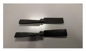
Fig. 6. 3D printed NACA proprotors.
