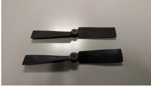
Fig. 6. 3D printed NACA propellers.
