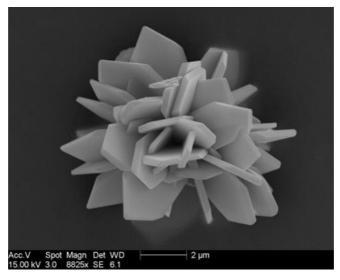
Fig 1 SEM image of the  $\beta(L)$ -Bi<sub>2</sub>Mo<sub>2</sub>O<sub>9</sub> phase.
