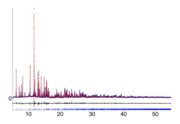
Fig. 2 Final Rietveld plot for  $\beta(L)$ -Bi<sub>2</sub>Mo<sub>2</sub>O<sub>9</sub>. The observed data are denoted by blue dot symbols, and the computed ones are represented by the continuous red line. The bottom line corresponds to the difference curve and the blue marks to the Bragg positions
