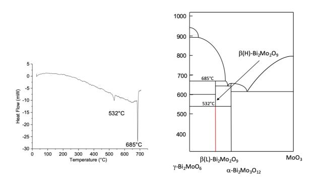
Fig 6 DTA analysis curve of the  $\beta(L)$ -Bi<sub>2</sub>Mo<sub>2</sub>O<sub>9</sub> phase recorded in air (10 mL min<sup>-1</sup>) at 5 °C min<sup>-1</sup>, and new phase diagram of the  $\gamma$ -Bi<sub>2</sub>MoO<sub>6</sub>-MoO<sub>3</sub> binary system.
