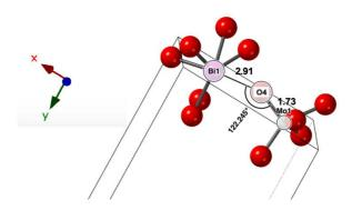
Fig. 8 Schematic representation of the proposed active site with selected geometries (Å) on the (101) surface of  $\beta(L)$ -Bi<sub>2</sub>Mo<sub>2</sub>O<sub>9</sub>.
