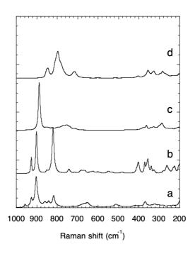
$\label{eq:Fig.7} \textbf{Fig. 7}: \mbox{ Raman spectra of the synthesized phases: (a)} \\ \gamma - \mbox{Bi}_2 \mbox{MoO}_6, (b) \\ \beta(\mbox{L}) - \mbox{Bi}_2 \mbox{Mo}_2 \mbox{O}_9, (c) \\ \beta(\mbox{H}) - \mbox{Bi}_2 \mbox{Mo}_2 \mbox{O}_9 \mbox{ and (d)} \\ \alpha - \mbox{Bi}_2 \mbox{Mo}_3 \mbox{O}_{12.} \\ \mbox{No}_3 \mbox$
