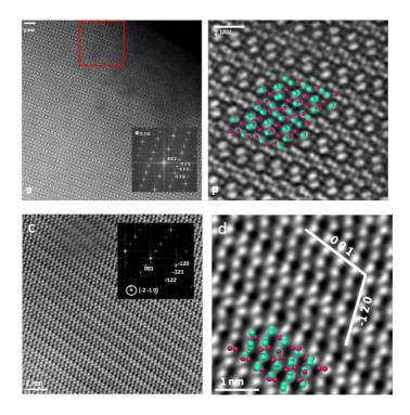
**Fig. 4** Atomic resolution HAADF image of the new phase, along the [110] zone axis (a,b) and the [-2-10] zone axis (c,d) at low-magnification. The indexed electron diffraction patterns (a and c) are shown at high-resolution, with a superimposed view of the computed schematic model (b and d).
