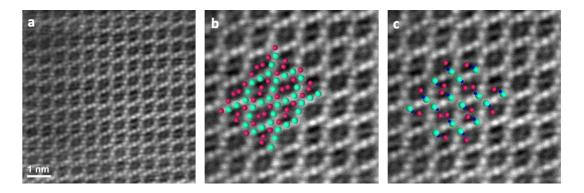
Fig. 9: HAADF STEM images of  $\beta(L)$ -Bi<sub>2</sub>Mo<sub>2</sub>O<sub>9</sub> in the (101) direction: a) bare structure, b) with bismuth (green) and molybdenum (red) atoms; c) with Bi(1), Mo(1) and O(4) (blue).
