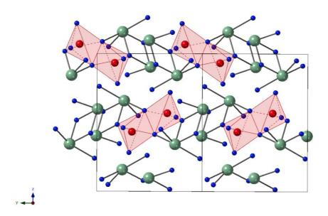
**Fig. 5** Projection of the structure of  $\beta(L)$ -Bi<sub>2</sub>Mo<sub>2</sub>O<sub>9</sub> along the *a* axis.
