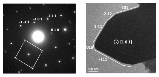
Fig. 3 TEM image of a platelet of  $\beta(L)$ -Bi<sub>2</sub>Mo<sub>2</sub>O<sub>9</sub> showing its faceting and the indexed electron diffraction pattern. A fluorite sub-cell is indicated by the dotted lines.
