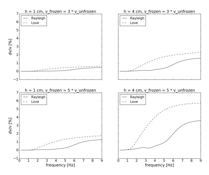
Figure 12: The results of four simulations with four different test models in the four subplots. The parameter h defines the thickness of the frozen layer.  $v_{frozen}$  is the shear wave velocity of the frozen layer and  $v_{unfrozen}$  is the velocity of the first layer (107 m s<sup>-1</sup>)
