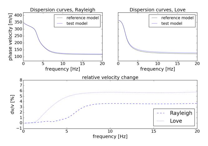
Figure 10: Results of dispersion curve modelling with Geopsy. Top left: dispersion curves of Rayleigh waves with test and reference model. Top right: dispersion curves of Love waves with test and reference model. Bottom: Ratio of the dispersion curves with test and reference model for Rayleigh and Love waves.
