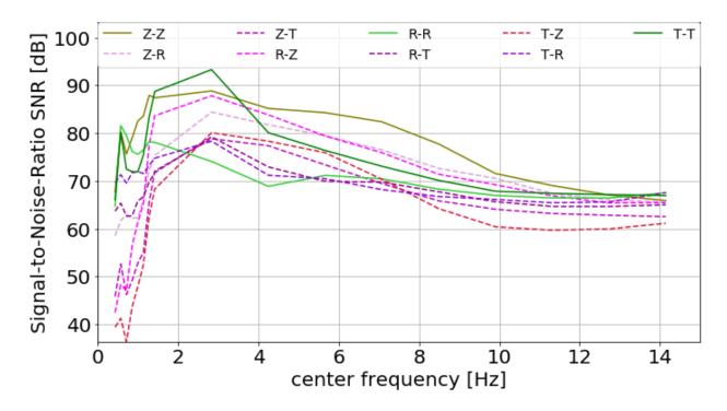
Figure 4: SNR depending on frequency averaged over causal and acausal side and all station pairs
