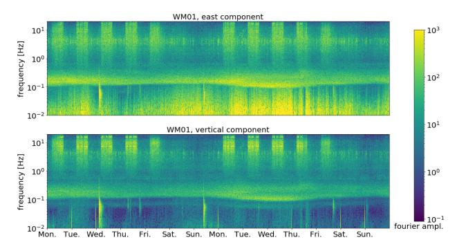
Figure 2: Spectrogram over two weeks starting at 8th of January 2018 for two components of WM01 with logarithmic frequency scale
