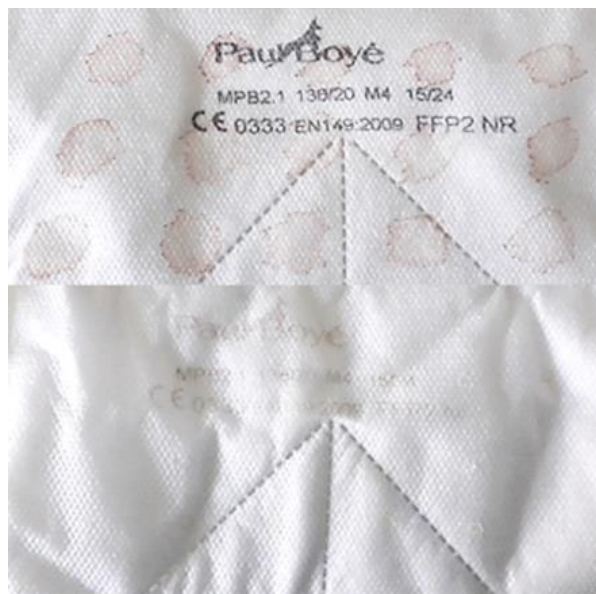
Figure 3: Pictures of FFP2 with serial dilution spores deposit (in the soiling solution composed of a mixture of erythrocytes and proteins) in triplicate, before (top) and after (bottom) SCCD treatment (343 K and 7.5 MPa for 1h).
