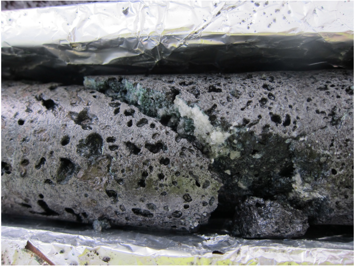
Fig 2: Basaltic core containing carbonates. The core was retrieved from about 450 m depth at the CarbFix pilot injection site in SW-Iceland in 2014 (photo: Sandra Snæbjörnsdóttir).
