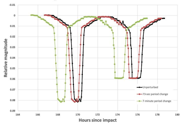
**Figure 5.** Schematic offset between the mutual events in the unperturbed Didymos system light curve and light curves from 73 s and 7-minute period changes, as seen 15 orbits following a leading-side ("head-on") DART impact. There is a roughly 18-minute difference between the timing of the mutual events of the unperturbed system and the minimum required 73 s period change case, easily detectable given expected data. The 7-minute period change leads to an even larger offset.
