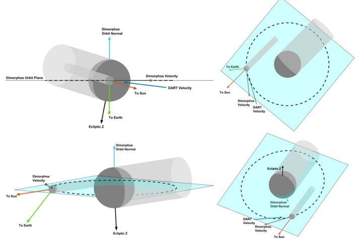
Figure 2. Geometry of DART Impact. Panels show the view from along the Didymos–Dimorphos line (top left), from above the system north pole (top right), from DART (bottom left), and from Earth (bottom right) at the final moments before the DART impact into Dimorphos. Included are the Dimorphos orbit plane and a schematic of the shadows cast by Didymos and Dimorphos.
