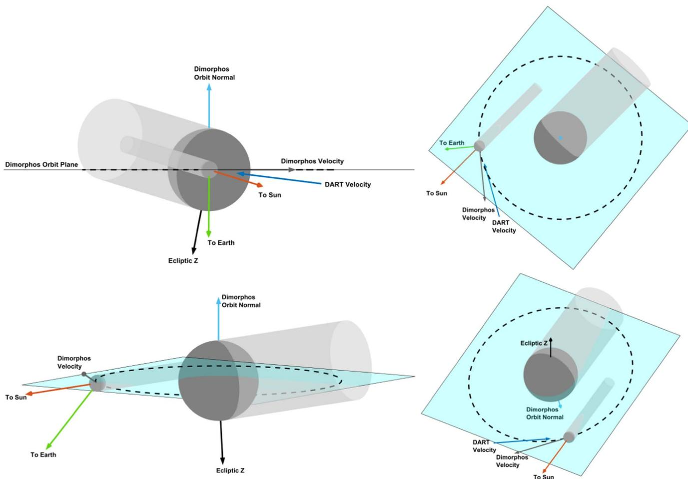
**Figure 2.** Geometry of DART Impact. Panels show the view from along the Didymos–Dimorphos line (top left), from above the system north pole (top right), from DART (bottom left), and from Earth (bottom right) at the final moments before the DART impact into Dimorphos. Included are the Dimorphos orbit plane and a schematic of the shadows cast by Didymos and Dimorphos.
