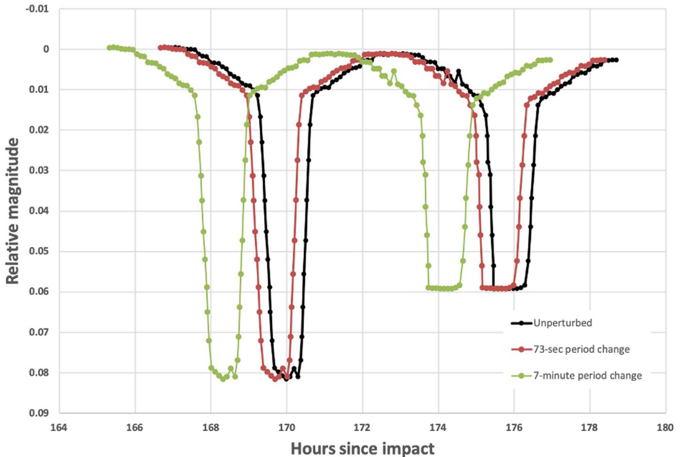
**Figure 5.** Schematic offset between the mutual events in the unperturbed Didymos system light curve and light curves from 73 s and 7-minute period changes, as seen 15 orbits following a leading-side (“head-on”) DART impact. There is a roughly 18-minute difference between the timing of the mutual events of the unperturbed system and the minimum required 73 s period change case, easily detectable given expected data. The 7-minute period change leads to an even larger offset.
