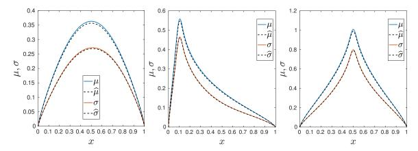
Figure 24: Case 4: direct estimates of  $\mu$  and  $\sigma$  and their regression surrogates  $\hat{\mu}$  and  $\hat{\sigma}$ ; distributed (left) and localized forcing at  $x_0 = 0.1$  (center) and  $x_0 = 0.5$  (right). In all cases,  $L_M = 0.573$ ,  $\sigma_M = 0.778$ , and  $\alpha = 0.5$ .
