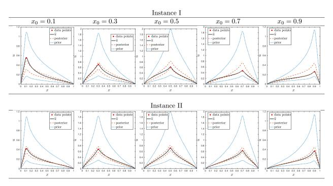
Figure 16: Case 2. Profiles of the solution, u, the 95% bounds of the pushed-forward prior (blue dash) and the 50% pushed-forward bounds of the posterior (red dash) of  $\xi$ . The plots correspond to localized forcing experiments as indicated. Top row: Instance I; bottom row: Instance II. The noisy measurements used in the inference are also depicted.
