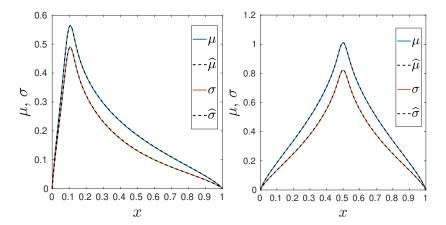
Figure 23: Case 4: profiles of  $\mu$  and  $\sigma$  compared to their surrogate predictions  $\widehat{\mu}$  and  $\widehat{\sigma}$ , for localized forcing at  $x_0=0.1$  (left) and  $x_0=0.5$  (right) and using  $L_M=0.573$ ,  $\sigma_M=0.778$  and  $\alpha=0.5$ .
