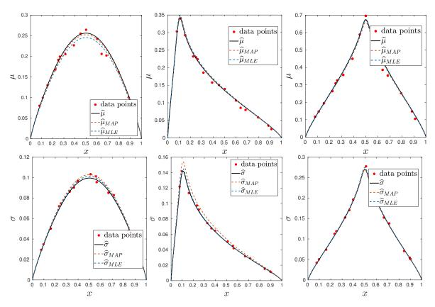
Figure 26: Case 4: MAP and MLE profiles of  $\mu$  (top) and  $\sigma$  (bottom) for distributed forcing (left) and localized forcing with  $x_0 = 0.1$  (center) and  $x_0 = 0.5$  (right). The true profiles are also plotted.
