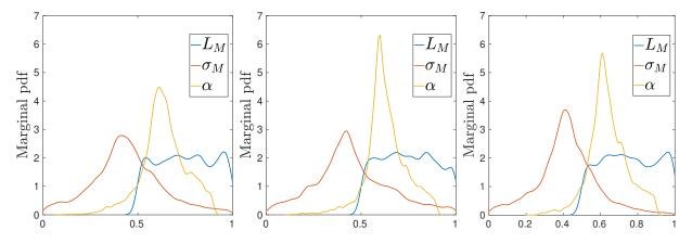
Figure 27: Case 4: marginal posterior pdfs of  $L_M$ ,  $\sigma_M$  and  $\alpha$  for distributed (left) and localized forcing at  $x_0 = 0.1$  (center) and  $x_0 = 0.5$  (right).
