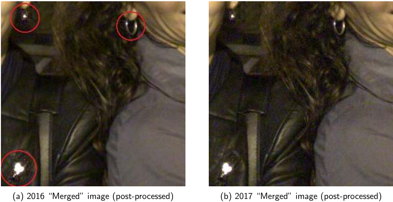
Figure 11: The Google 2016 results seem to feature less residual noise except around strong high contrast features / specular highlights, which is typical of spatial denoising as stated in [9].
