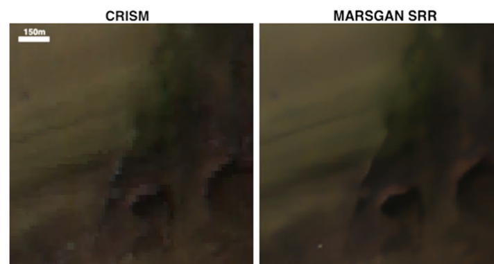
Figure 22. Comparison of the 18 m/pixel CRISM image (frt0000d3a4_07_if164l_trr3_raw; using band 233, band 78, and band 13 for RGB colour) and the MARSCHAN SRR result over Capri Chaos, Valles Marineris.
