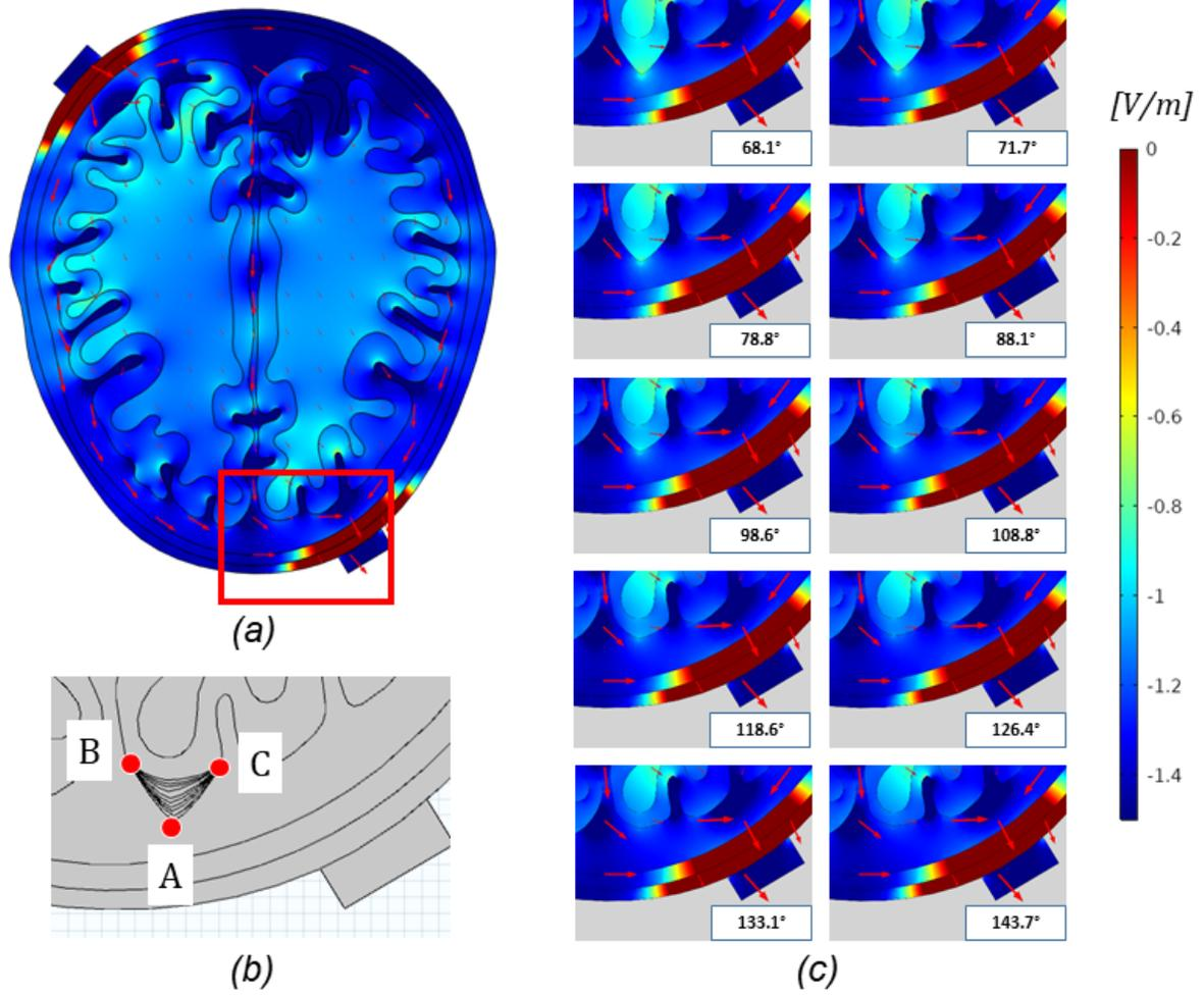
Figure 2. (a) Electric field distribution on the global surface with an input current of 2mA at 1 kHz; (b) Variation of the wedge angle  $\theta$  from  $68^\circ$  to  $143^\circ$ ; and (c) Associated electric field distribution.
