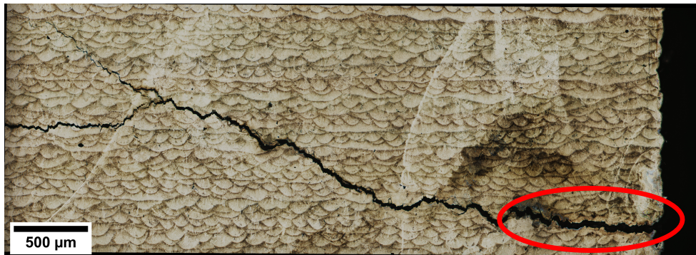
Figure 4: A crack in an H13 sample observed after a chemical etching with Fry's reagent. Delamination is visible in the red circle.
