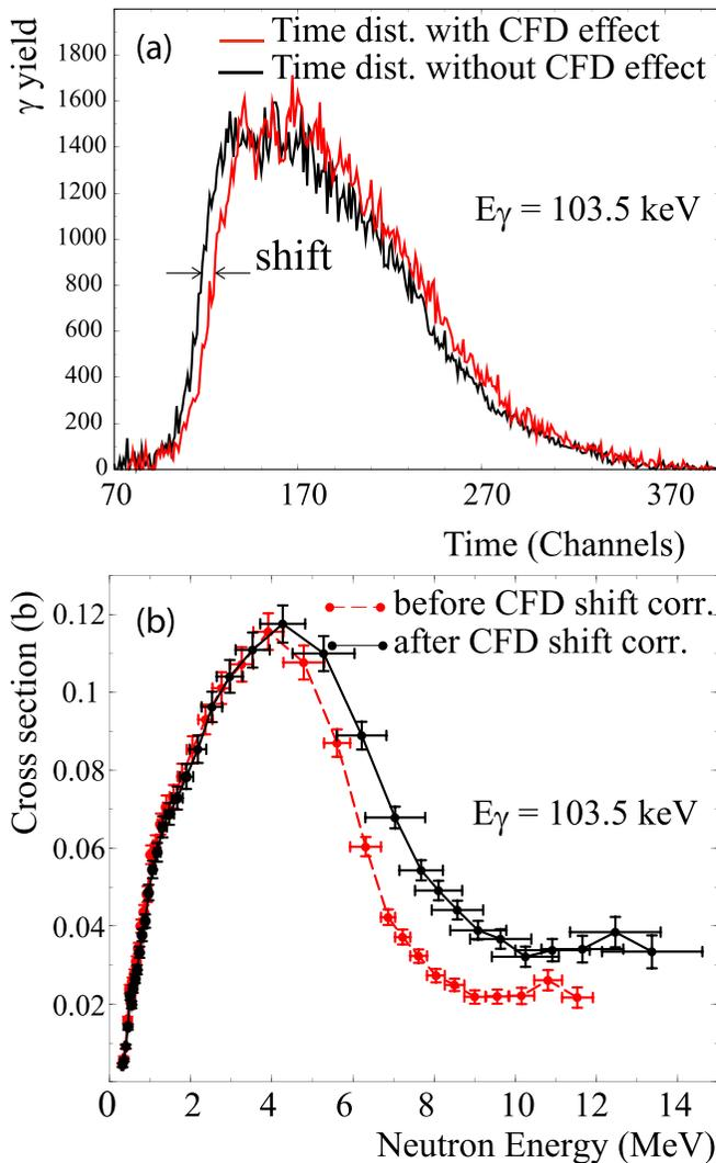
FIG. 6. (a) Time distributions for the detector G110 and for  $\gamma$  energy at 103.5 keV. The black distribution is not affected by CFD shift while the red one is. These two distributions are used to define the time correction to apply to the data for each impacted  $\gamma$  transition. (b) Cross section data for the 103.5-keV  $\gamma$  transition before the CFD shift correction (in red) and after (in black).
