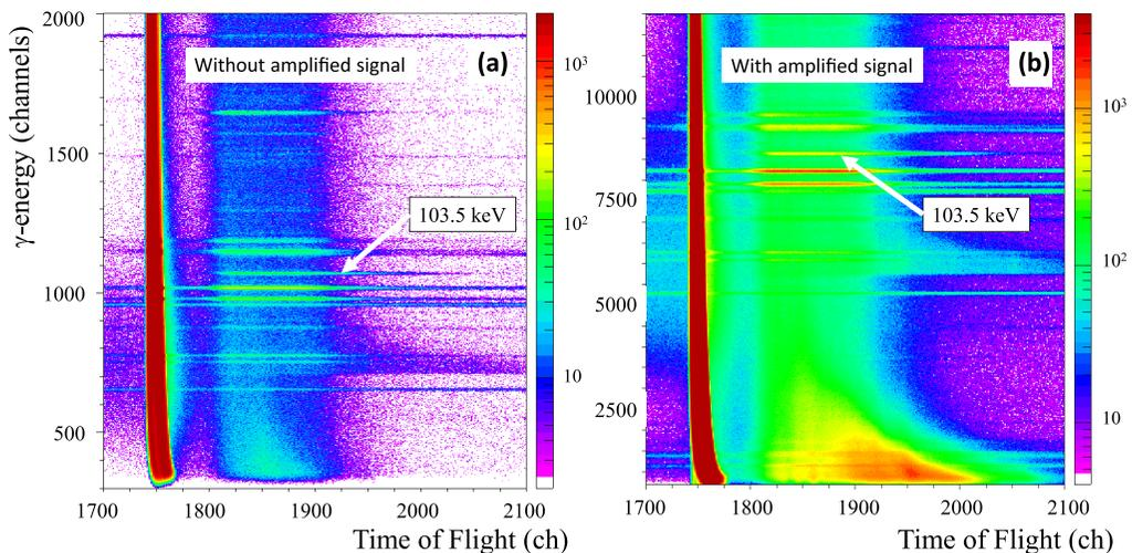
FIG. 5. Zoomed-in look of the time-amplitude matrix corresponding to the low-energy  $\gamma$  lines with unamplified (a) and amplified (b) signals. The so-called “walk” effect is clearly visible in panel (a).
