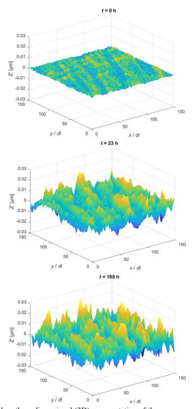
**Figure 3** Exemplary three-dimensional (3D) representation of the mean-removed topography data, Z', (see Section 2.2) associated with a selected sample window, after replacement of 'dead pixels' and VSI-related artifacts (see Section 2.1.5), and second order degree de-trending at observation times t = 0, 23, and 188 hours.
