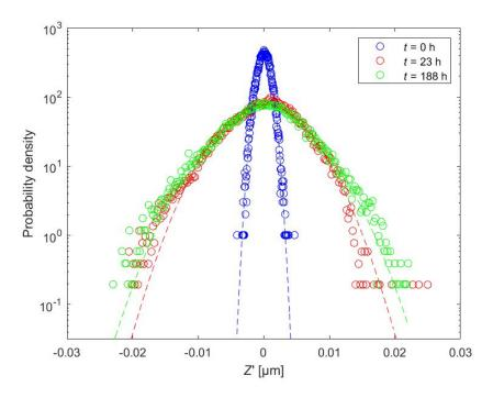
**Figure 4** Comparison of the sample distributions probability densities of the variable Z' at observation times t = 0, 23, and 188 hours (open circles) with Gaussian distributions densities (dashed lines) characterized by the same mean and standard deviation of Z'. The distribution of Z' appears to be symmetric at t = 0 hours and slightly asymmetric (left-skewed) at longer times.
