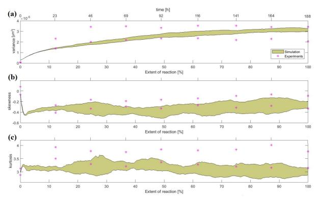
**Figure 9** Temporal evolution of the key statistics of Z' evaluated over 100 realizations of *Model 3*. Envelopes of width equal to  $\pm$  one standard deviation around the corresponding mean are depicted (shaded areas). Symbols denote the corresponding intervals associated with the experimental data monitored across the 9 sample windows investigated.
