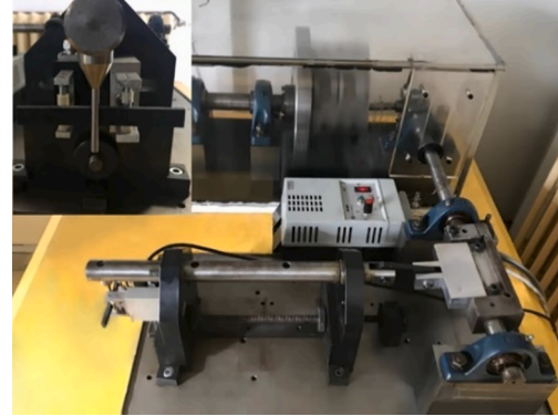
Fig. 5. The mechanical system of the three-point bending fatigue test apparatus.
