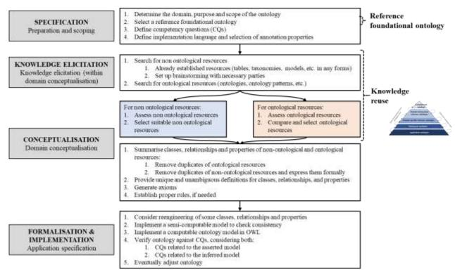
Figure 2 – AMODO methodology for ontology modelling.
