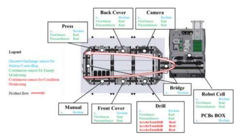
Figure 8 – Laboratory layout with indications on sensors installation.
