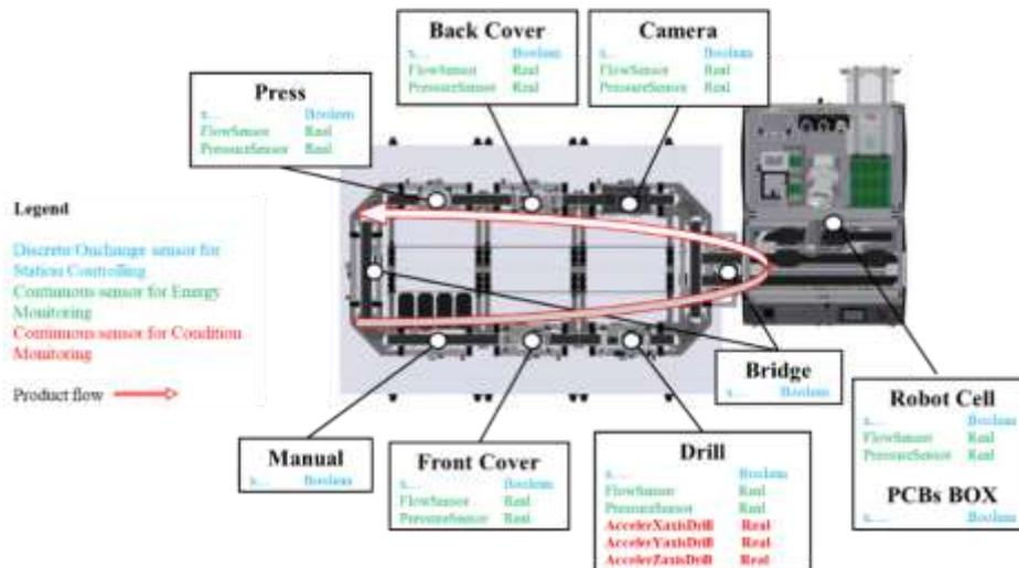
Figure 8 – Laboratory layout with indications on sensors installation.
