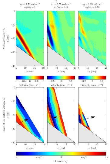
FIGURE 10. The components of the inertial wave field (displayed in terms of the vertical velocity component) filtered at frequencies  $\omega_0$ ,  $\omega_1$  and  $\omega_2$  (upper row), with the corresponding phase patterns (lower row). Only one branch of the wave attractor is shown. The corresponding vector triad is shown in figure 12 (a).
