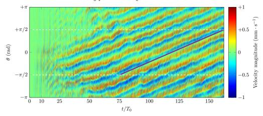
FIGURE 5. Temporal evolution of the radial velocity as a function of azimuth,  $\theta$ , obtained by taking profiles of radial velocity at radius r=8 cm in the horizontal plane at  $\simeq 20$  cm depth. To guide the eye, we added a solid line showing that the cluster rotates half a turn ( $\pi$  rad) in  $(88 \pm 2)T_0$ .
