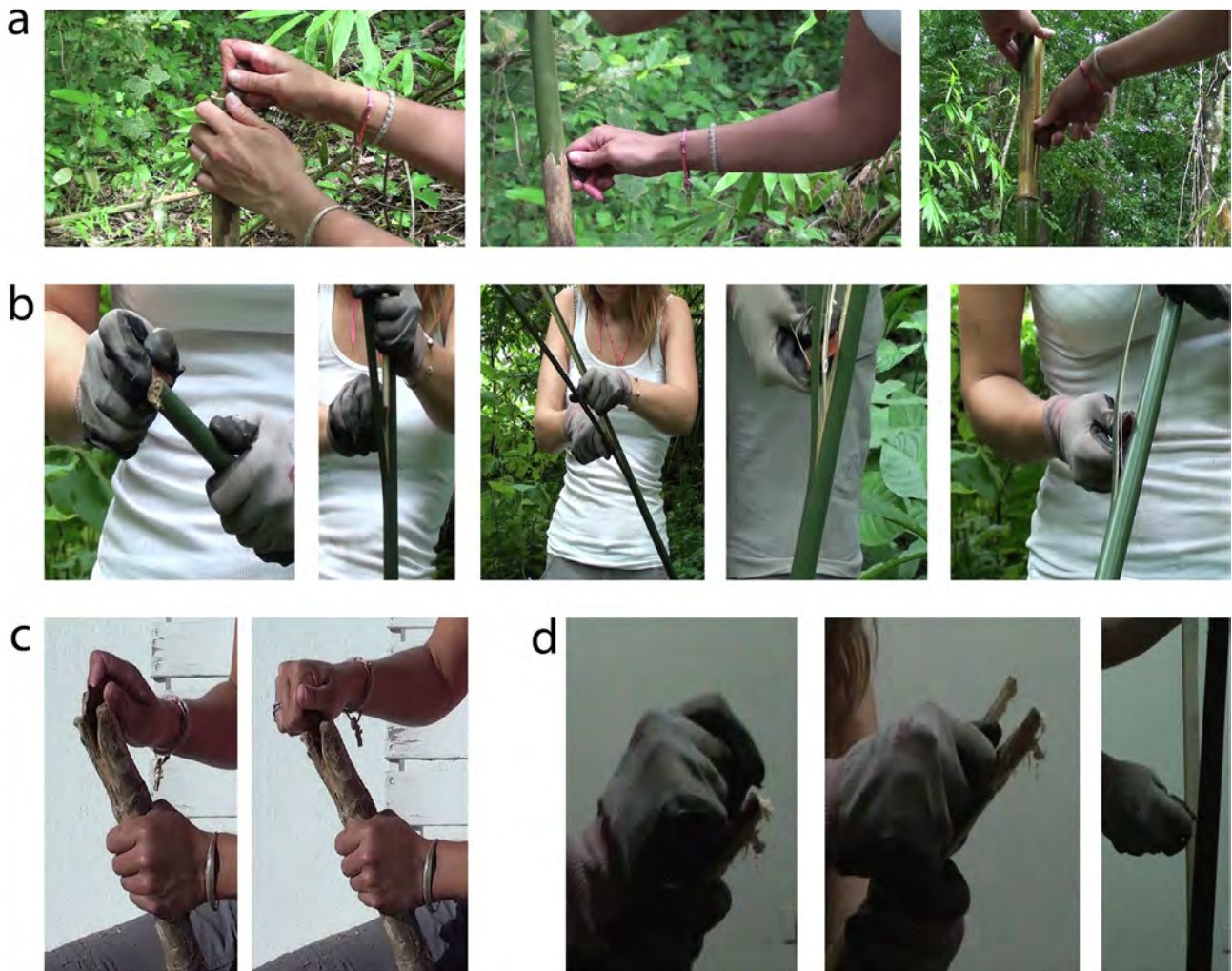
Fig. 5. Examples of plant splitting experiments. a) Bamboo culms ( Schizostachyum cf. lima ) b) Stems of Donax cannaeformis . c) Rattan stem ( Calamus merrillii ) d) Long palm leaf petioles ( Arenga pinnata ).
