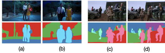
Figure 5. Examples of frame layering. (top) Raw frames, and (bottom) layer maps with overlaid character segmentation masks. Our pipeline (a), (b): correctly predicts the number of layers and is consistent over time. (c), (d): incorrectly predicts a new layer (purple) when a character moves towards the background.
