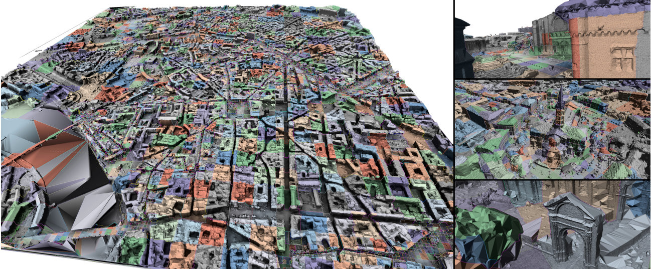
Figure 8: Reconstruction result on a 350 million points data set. Tiling is visualised through a random color per tile.
