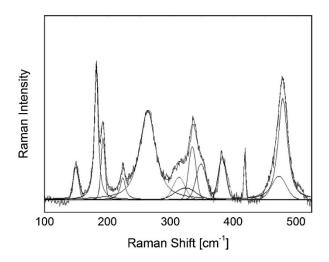
**Figure 1.** Example of a fitted Raman spectrum of Delta using the procedure followed in this paper. The spectrum was taken on a head specimen in a region with a high monoclinic fraction.
