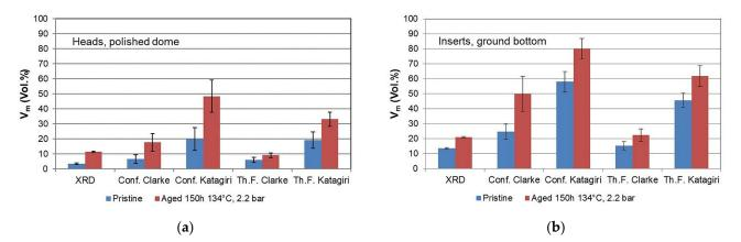
**Figure 2.** Values of  $V_m$  measured by Raman spectroscopy and XRD on both non-aged and in vitro aged Delta heads (**a**) and inserts (**b**). Conf. = confocal pinhole closed down to 100 µm (penetration depth of Raman signal: 4.2 µm); Th. F. = confocal pinhole fully open (1000 µm)—penetration depth of Raman signal: 15 µm.
