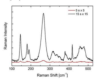
**Figure 6.** Raman spectra collected on Delta with different acquisition times in order to obtain different SNRs. The spectra were collected on the same point of a polished specimen surface, but the low-SNR spectrum mimics the case of a spectrum collected through a metal layer in correspondence with metal transfer.
