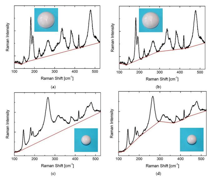
**Figure 7.** Different baseline choices on Raman spectra of Delta with (**a**,**b**) high and (**c**,**d**) low monoclinic contents. The spectrum shown in (**a**,**b**) was collected on the rear of an insert (rough surface), whereas the spectrum shown in (**c**,**d**) was collected on the apex of a head (polished surface).
