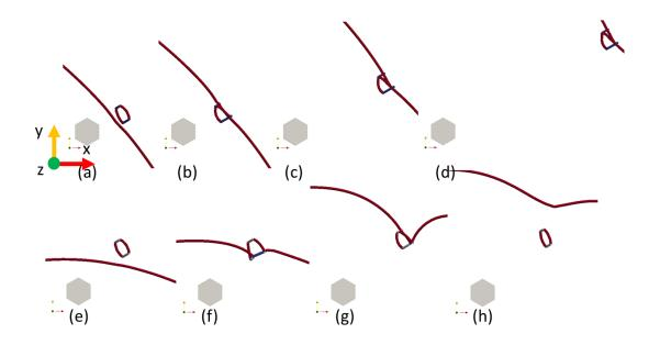
Figure 7 : Sequence showing an interaction between a mixed dislocation of Burgers vector  $\underline{b}_G = \underline{b}_2$  gliding in the basal plane and a loop with Burgers vector  $\underline{b}_L = \underline{b}_3$ . (a), (b), (c), (d)  $\theta$ =54°: no pinning, significant clearing. (e) (f) (g) (h)  $\theta$ =84°: strong pinning, no clearing.
