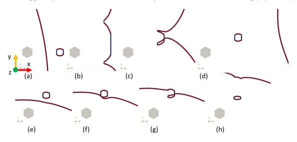
Figure 5 : Sequence showing an interaction between a mixed dislocation of Burgers vector  $\underline{b}_G = \underline{b}_2$ gliding in the basal plane and a loop with Burgers vector  $\underline{b}_L = \underline{b}_2$ . (a), (b) (c) (d)  $\theta$ =10°: strong pinning, no clearing. (e) (f) (g) (h)  $\theta$ =84°: partial clearing, no pinning.
