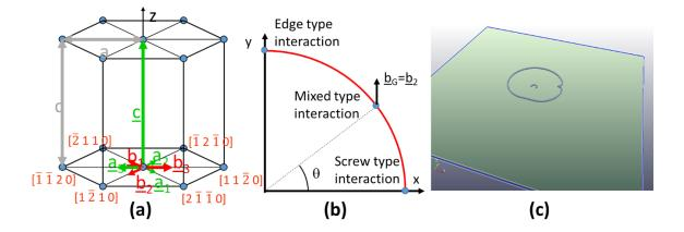
Figure 1 : (a) 4-indices Miller-Bravais convention for HCP structure. (b) Schematic describing the systematic study of interactions between mixed dislocations and loops. (c) Snapshot of the simulation box showing the interaction between a loop and a dislocation with the same Burgers vector ( $\theta$ =10°).
