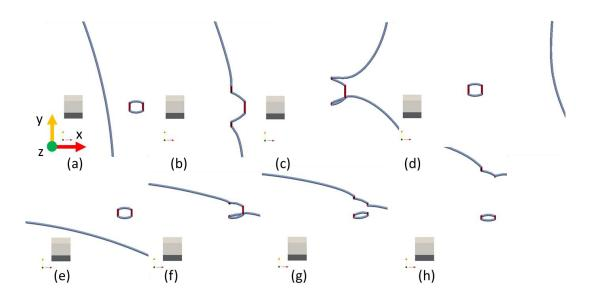
Figure 2 : Sequence showing an interaction between a mixed dislocation of Burgers vector  $\underline{b}_G = \underline{b}_2$  gliding in the prismatic plane and a loop with Burgers vector  $\underline{b}_L = \underline{b}_2$ . (a), (b), (c), (d)  $\theta$ =10°: strong pinning, no clearing. (e) (f) (g) (h)  $\theta$ =72°: partial clearing, no pinning.
