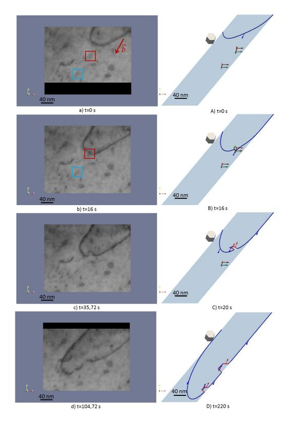
Figure 9 : Incorporation case. a) to d) In situ observation in a TEM of a dislocation interacting with a loop. A) to D) DD simulation of the dislocation – loop interaction.
