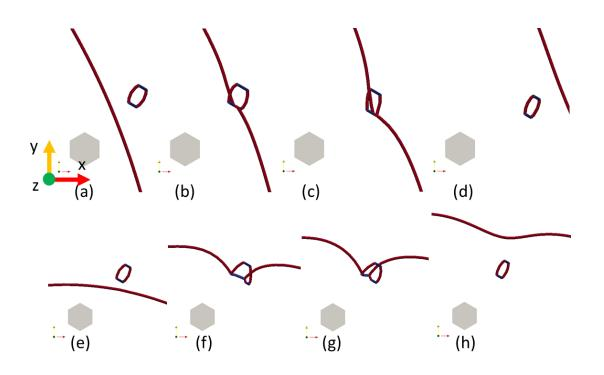
Figure 6 : Sequence showing an interaction between a mixed dislocation of Burgers vector  $\underline{b}_G = \underline{b}_2$  gliding in the basal plane and a loop with Burgers vector  $\underline{b}_L = \underline{b}_1$ . (a), (b), (c) (d)  $\theta$ =32°: no pinning, no clearing. (e), (f), (g), (h)  $\theta$ =84°: strong pinning, no clearing.
