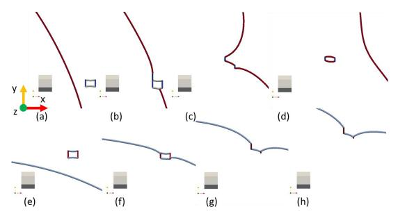
Figure 3 : Sequence showing an interaction between a mixed dislocation of Burgers vector  $\underline{b}_G = \underline{b}_2$  gliding in the prismatic plane and a loop with Burgers vector  $\underline{b}_L = \underline{b}_1$ . (a), (b), (c), (d)  $\theta$ =21°: strong pinning, no clearing. (e), (f), (g), (h)  $\theta$ =72°: full clearing, no pinning.
