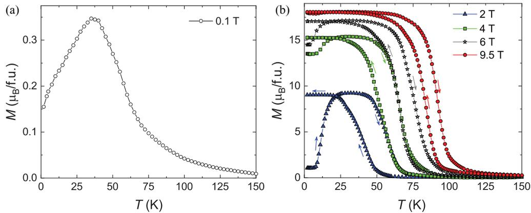
FIG. 3. Temperature dependence of the magnetization of  $\text{La}_{0.85}\text{Ce}_{0.15}\text{Fe}_{12}\text{B}_6$ : (a) magnetization measured using zero-field cooled (ZFC) protocol in 0.1 T applied magnetic field; (b) magnetization measured in applied magnetic fields of 2, 4, 6, and 9.5 T [both ZFC and field cooled (FC) data are marked by the same symbols]. The arrows indicate the direction of the temperature change.
