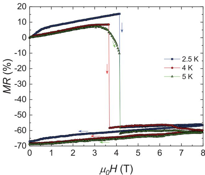
FIG. 7. Magnetic field dependence of the isothermal magnetoresistance of  $\text{La}_{0.85}\text{Ce}_{0.15}\text{Fe}_{12}\text{B}_6$  measured at 2.5, 4 and 5 K.
