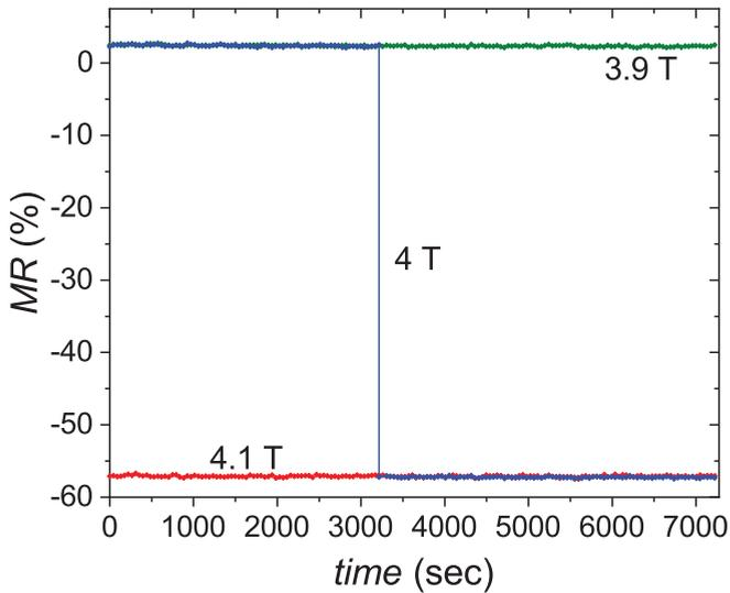
FIG. 10. Time dependence of the magnetoresistance recorded at the indicated applied fields for  $\text{La}_{0.85}\text{Ce}_{0.15}\text{Fe}_{12}\text{B}_6$  at 2.5 K.
