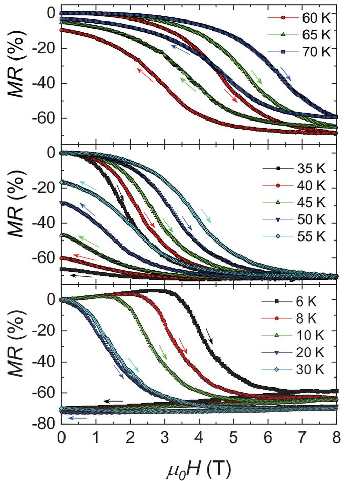
FIG. 8. Magnetoresistance isotherms of  $\text{La}_{0.85}\text{Ce}_{0.15}\text{Fe}_{12}\text{B}_6$  at the indicated temperature ranging from 6 to 30 K (bottom panel), 35 to 55 K (middle panel) and 60 to 70 K (top panel).
