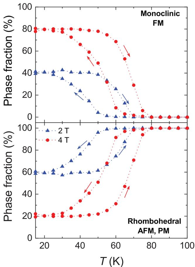
FIG. 15. Temperature dependence of the phase fractions of both rhombohedral and monoclinic crystal structures of  $\text{La}_{0.85}\text{Ce}_{0.15}\text{Fe}_{12}\text{B}_6$  as determined from x-ray powder diffraction measurements during heating and cooling in  $\mu_0H = 2$  and 4 T applied magnetic fields.
