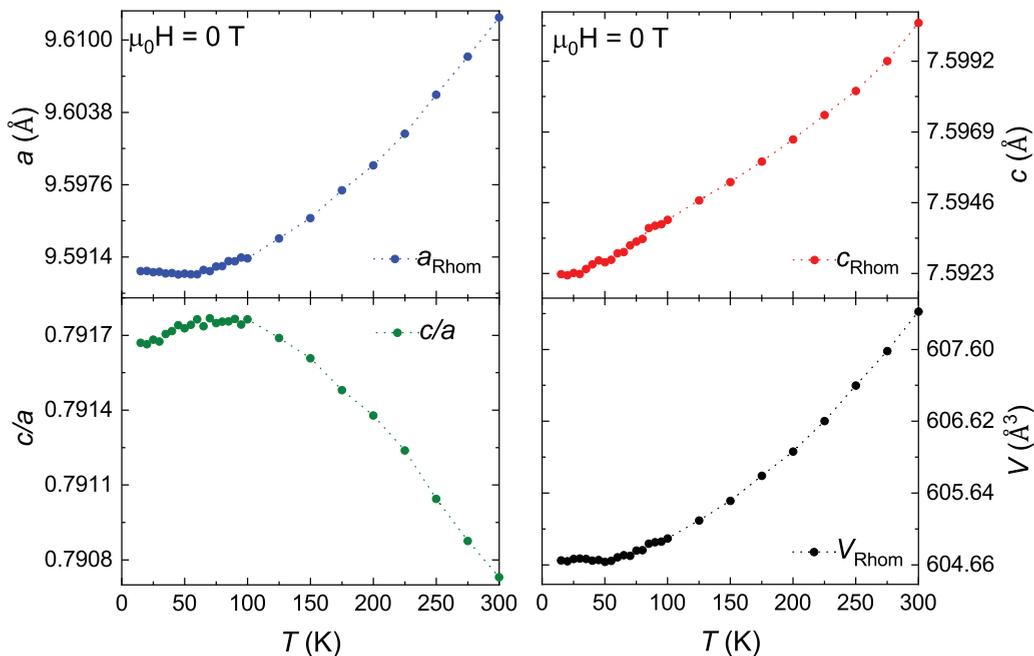
FIG. 2. Temperature dependence of the lattice parameters  $a$  and  $c$ ,  $c/a$  ratio, and unit cell volume  $V$  of the rhombohedral cell for  $\text{La}_{0.85}\text{Ce}_{0.15}\text{Fe}_{12}\text{B}_6$  as derived from Rietveld refinement of the diffraction patterns collected upon cooling in  $\mu_0H = 0$  T. Dashed lines are guide for the eye.
