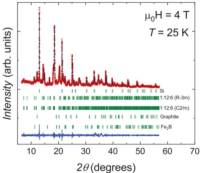
FIG. 12. Rietveld refinement of the x-ray powder diffraction pattern collected at 25 K in magnetic field of  $\mu_0 H = 4$  T for the  $\text{La}_{0.85}\text{Ce}_{0.15}\text{Fe}_{12}\text{B}_6$  compound. The observed (red dots) and calculated (black lines) patterns are shown. The blue line represents the difference  $I_{\text{obs}} - I_{\text{calc}}$ . The vertical bars (olive) indicated positions of Bragg peaks for the different phases.
