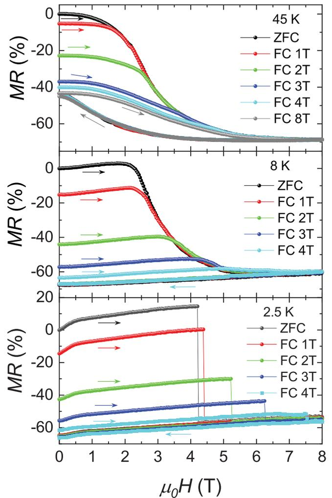
FIG. 9. Isothermal magnetoresistance of  $\text{La}_{0.85}\text{Ce}_{0.15}\text{Fe}_{12}\text{B}_6$  at some selected temperatures of 2.5 K (bottom panel), 8 K (middle panel), and 45 K (top panel) taken after cooling the sample in different magnetic fields.
