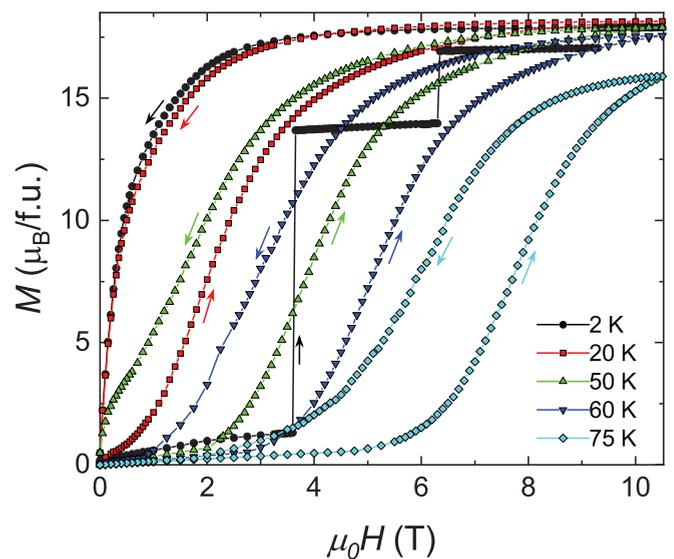
FIG. 4. Magnetization isotherms of  $\text{La}_{0.85}\text{Ce}_{0.15}\text{Fe}_{12}\text{B}_6$  measured between 2 and 75 K.
