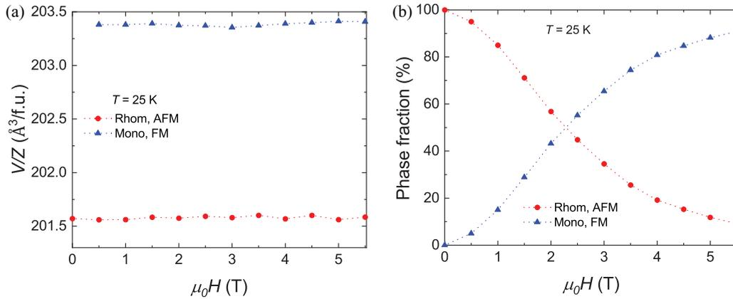
FIG. 18. Magnetic field dependence of the (a) cell volume per chemical formula for  $\text{La}_{0.85}\text{Ce}_{0.15}\text{Fe}_{12}\text{B}_6$  and (b) phase fractions of both rhombohedral and monoclinic crystal structures determined from x-ray powder diffraction measurements at 25 K.
