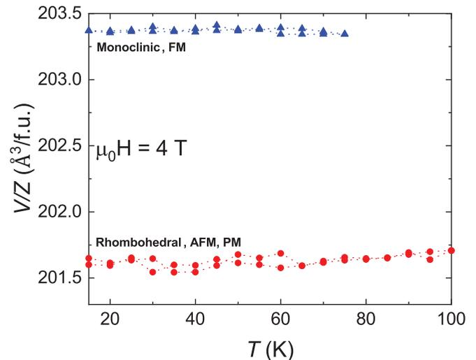
FIG. 13. Temperature dependence of the cell volume per formula unit for  $\text{La}_{0.85}\text{Ce}_{0.15}\text{Fe}_{12}\text{B}_6$  (both rhombohedral and monoclinic phases) derived from x-ray diffraction measurements during heating and cooling in  $\mu_0 H = 4$  T applied magnetic field.
