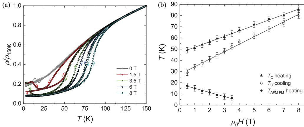
FIG. 6. (a) Temperature dependence of the relative electrical resistivity of  $\text{La}_{0.85}\text{Ce}_{0.15}\text{Fe}_{12}\text{B}_6$  on heating and cooling in various applied magnetic fields. Both zero-field cooled (ZFC) and field cooled (FC) data are marked by the same symbols. The arrows indicate the direction of the temperature change. (b) Magnetic field dependence of the transition temperatures.
