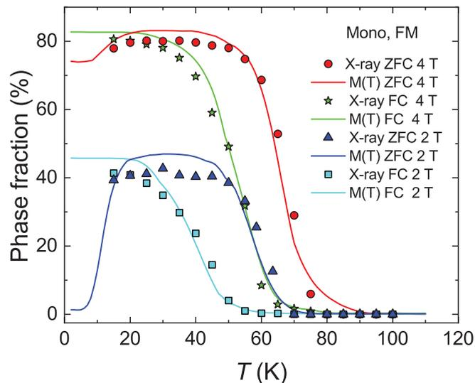
FIG. 17. Temperature dependence of the concentration of the monoclinic phase of  $\text{La}_{0.85}\text{Ce}_{0.15}\text{Fe}_{12}\text{B}_6$  as determined from x-ray powder diffraction (symbols) and magnetization (lines) measurements during heating and cooling in  $\mu_0H = 2$  and 4 T fields.
