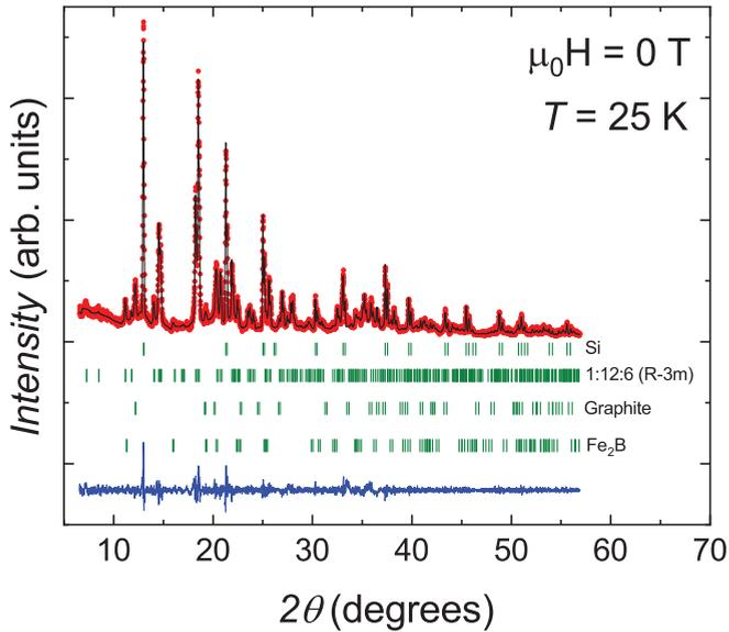
FIG. 1. Rietveld refinement of the x-ray powder diffraction pattern collected at 25 K in  $\mu_0H = 0$  T for the  $\text{La}_{0.85}\text{Ce}_{0.15}\text{Fe}_{12}\text{B}_6$  compound. The observed (red dots) and calculated (black lines) patterns are shown. The blue line represents the difference  $I_{\text{obs}} - I_{\text{calc}}$ . The vertical bars (olive) indicate positions of Bragg peaks for the different phases.
