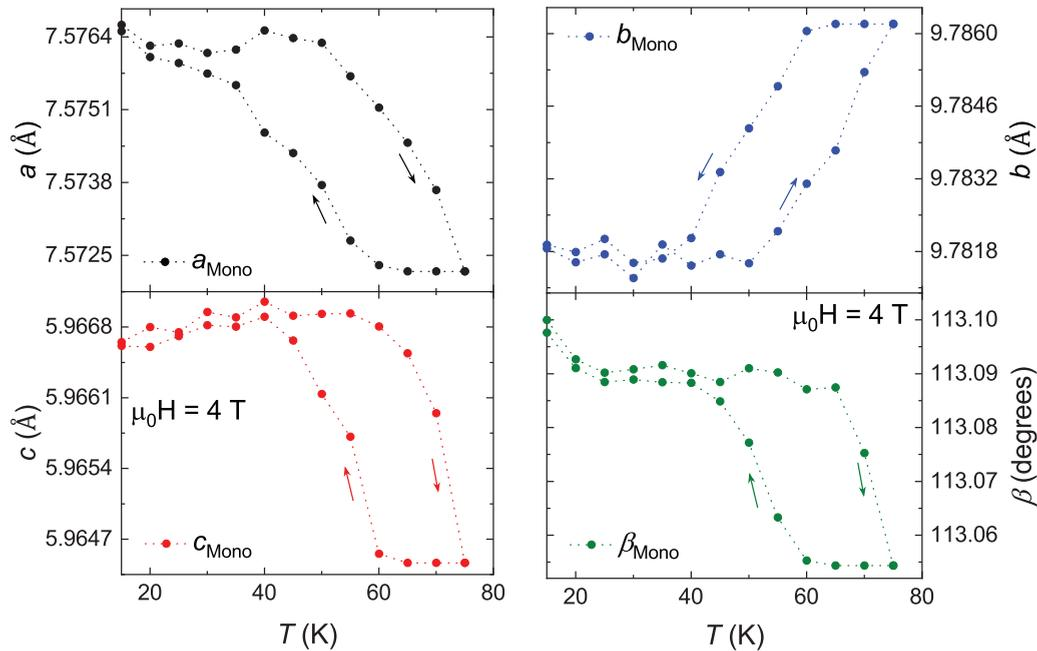
FIG. 14. Temperature dependence of the lattice parameters  $a$ ,  $b$ , and  $c$ , and Bragg angle  $\beta$  of the monoclinic phase determined from x-ray powder diffraction measurements during heating and cooling in  $\mu_0 H = 4$  T applied magnetic field.
