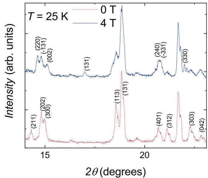
FIG. 11. Diffraction patterns measured at 25 K in magnetic fields of 0 and 4 T for the  $\text{La}_{0.85}\text{Ce}_{0.15}\text{Fe}_{12}\text{B}_6$  compound. Only the low angle part (from  $14^\circ$  to  $23^\circ$ ) of the diffraction pattern is shown to better illustrate development of phases with applied magnetic field.
