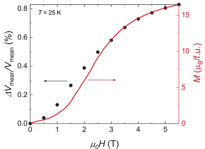
FIG. 20. Magnetic field dependence of the relative volume change and the magnetization at 25 K of  $\text{La}_{0.85}\text{Ce}_{0.15}\text{Fe}_{12}\text{B}_6$ .
