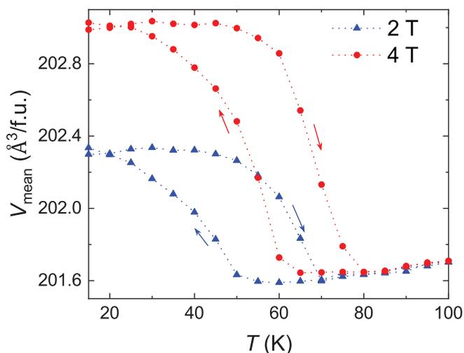
FIG. 16. Temperature dependence of the mean cell volume per formula unit determined from x-ray powder diffraction measurements during heating and cooling in  $\mu_0H = 2$  and 4 T applied magnetic fields.
