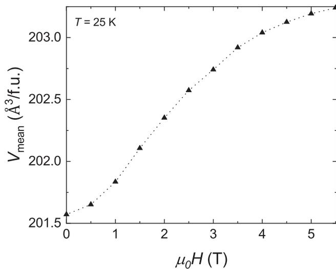
FIG. 19. Magnetic field dependence of the mean cell volume per chemical formula determined from powder diffraction measurements at 25 K for  $\text{La}_{0.85}\text{Ce}_{0.15}\text{Fe}_{12}\text{B}_6$ .
