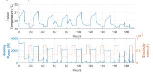
Figure 8: Optimisation combining the GSHP and building model
