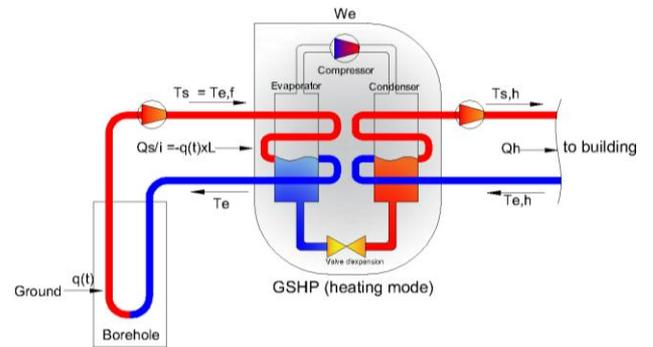
Figure 4: Ground Source Heat Pump model
