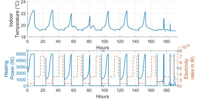
Figure 5: Optimisation of electric heater for one week
