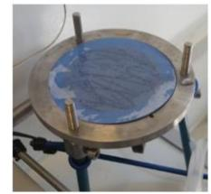
Figure 4: Open filtration tripod with a filter membrane placed on it.
