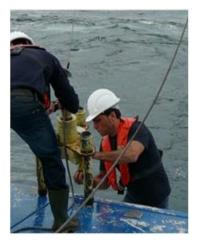
Figure 8: Multicorer deployment in an intertidal area.
