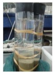
Figure 9: Example of corers that contain soft sediment and overlaying seawater.
