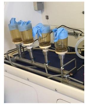
Figure 6: Set up of the WaSOP 2 and WaSOP 3 filtration equipment (filtration ramp and 47 mm filtration units) on the laboratory bench. The filtration system is connected to a vacuum pump and filtration takes place in parallel in the 4 filtration units.
