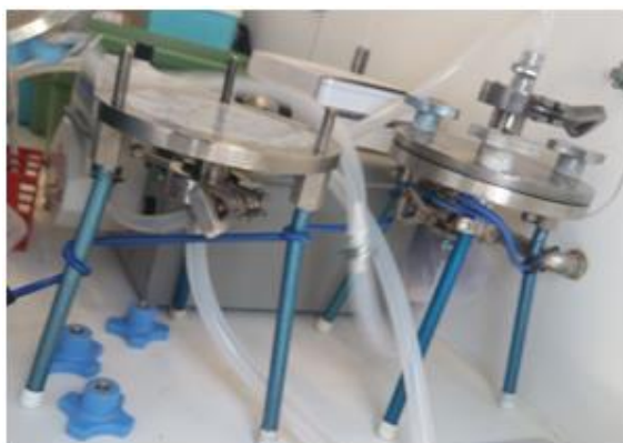
Figure 5: Open (left) and close (right) filtration tripods.
