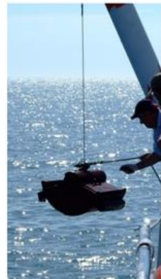
Figure 10: Grab deployment from a RV.
