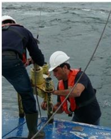
Figure 8: Multicorer deployment in an intertidal area.
