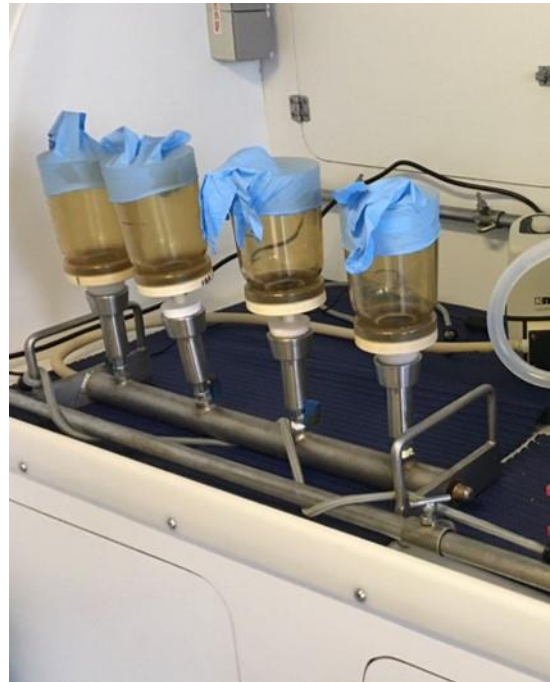
Figure 6: Set up of the WaSOP 2 and WaSOP 3 filtration equipment (filtration ramp and 47 mm filtration units) on the laboratory bench. The filtration system is connected to a vacuum pump and filtration takes place in parallel in the 4 filtration units.
