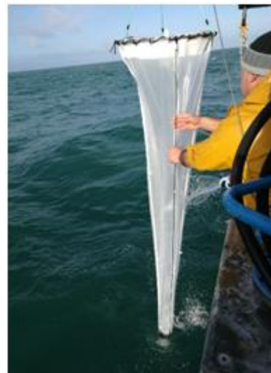
Figure 7: Vertical tow onboard a RV. The WP2 net is clean and about to be towed.
