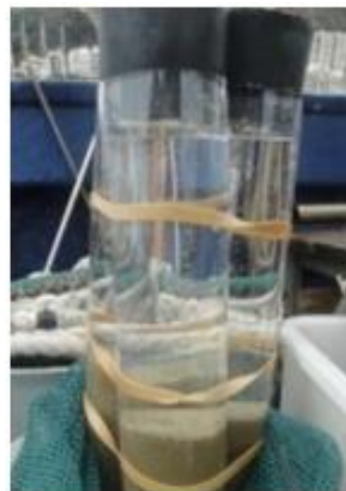
Figure 9: Example of corers that contain soft sediment and overlaying seawater.
