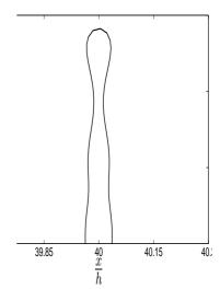
FIGURE 1 – Left: Rundown for soliton of initial amplitude a/h=0.7. Free surface elevation at several instants of time. (····)  $t/\tau=16$ , (- - -)  $t/\tau=17$ , and (o)  $t/\tau=18$ . Residual falling jet for initial amplitude a/h=0.7 at time  $t/\tau=18$ .
