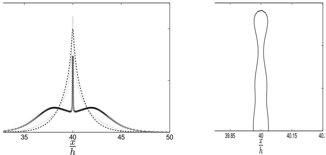
FIGURE 1 – *Left* : Rundown for soliton of initial amplitude  $a/h = 0.7$ . Free surface elevation at several instants of time. (····)  $t/\tau = 16$ , (- - -)  $t/\tau = 17$ , and (○)  $t/\tau = 18$ . *Right* : Residual falling jet for initial amplitude  $a/h = 0.7$  at time  $t/\tau = 18$ .
