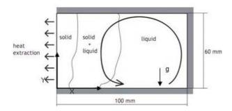
FIG. 1 - Schematic of the 2D side-cooled solidification problem
