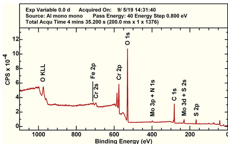
Fig. 1. Survey spectrum obtained for molybdenum sulfate sample.
