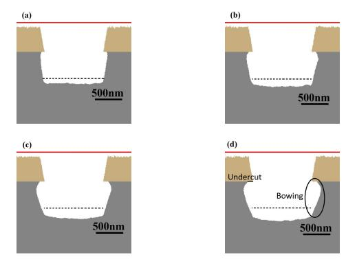
**Figure 13.** Trenches profiles determined by modeling for different reflection probability for  $Cl \to FeCl_x(x=0-2)$  reactions: (a)  $P_{ads}=0.1$ , (b)  $P_{ads}=0.2$ , (c)  $P_{ads}=0.3$  and (d)  $P_{ads}=0.4$ . Etching time is 2 min, other operating conditions are presented in table 3. Dashed lines represent etching depth estimated with experimental etch rate for pure iron sample.
