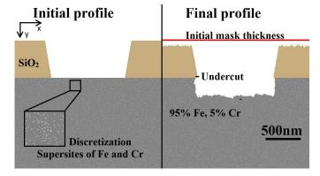
**Figure 2.** Initial and final profile provided by surface model during Fe/Cr etching using pure  $Cl_2$  plasma.
