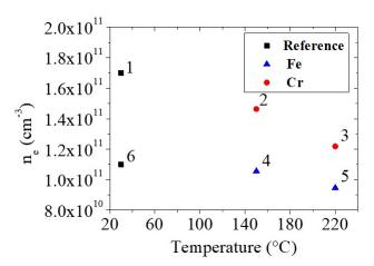
Figure 12. Electron density of  $Cl_2$  plasmas for conditions presented in table 3 with different substrate temperatures (150  $^{o}C$  for points 2 and 4, 220 $^{o}C$  for points 3 and 5). References of  $n_e$  given by points 1 and 6 (without substrate heating), before any etching (point 1) and after every etching (point 6).
