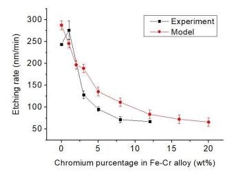
**Figure 14.** Experimental and modeling etch rates of Fe/Cr target with different %Cr. Operating conditions are presented in table 3.
