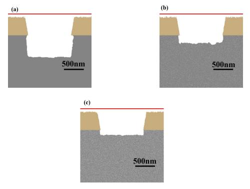
**Figure 15.** Trenches profiles determined by modeling for : (a)  $0 \% wt \ Cr$ , (b)  $8\% wt \ Cr$  and (c)  $20\% wt \ Cr$ . Etching time is  $2 \ min$ , other operating conditions are presented in table 3
