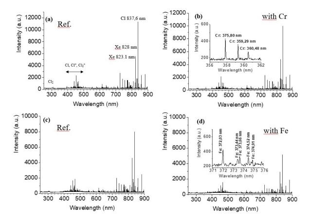
**Figure 11.** Emission spectra of a chlorine plasma. Pressure is 5 mTorr, RF Power is 800 W,  $Cl_2$  flow rate is 60 sccm Xe flow rate is 7 sccm with neither bias, nor sustrate heating. There is a Cr metallic substrate for figure b and a Fe metallic substrate for figure d.
