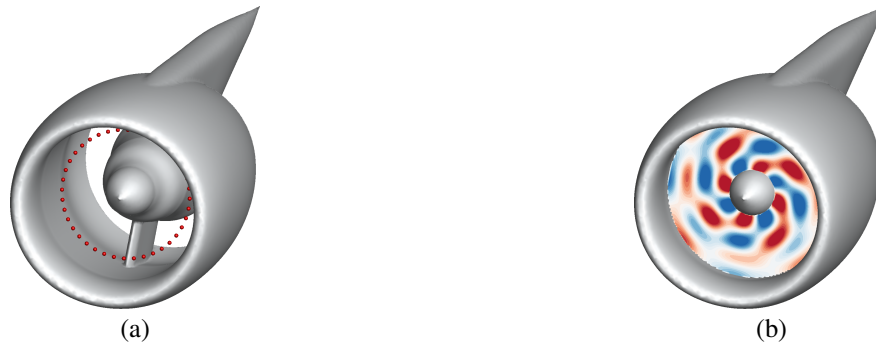
Fig. 5 Views of (a) monopoles position inside the nacelle and (b) instantaneous pressure field generated in the source plane
