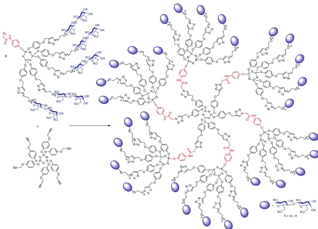
**Scheme 6.** Synthesis of a layered onion peel dendrimer by click chemistry, starting from a dendron bearing lactoside terminal functions. The deprotection of the carbohydrate is carried out in the last step.
