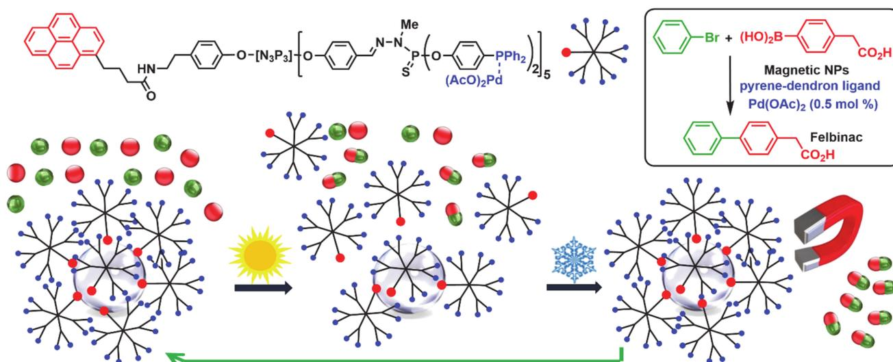
**Scheme 12.** Non-covalent grafting of catalytic dendrons onto cobalt nanoparticles covered by graphene layers, and their use as catalysts in Suzuki couplings. Example of coupling for the synthesis of Felbinac. Recovering and re-use were carried out eleven times, with a quantitative yield in Felbinac in all cases.
