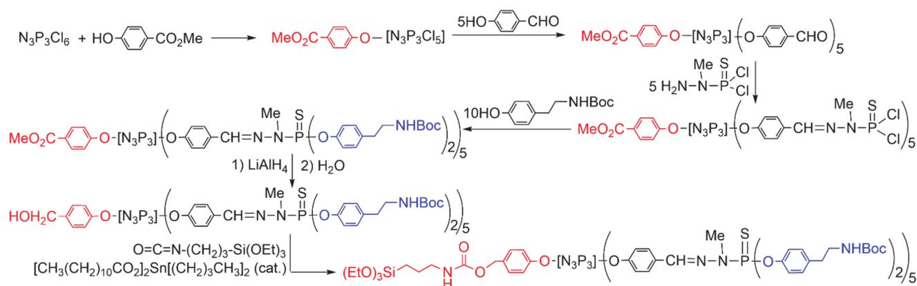
**Scheme 11.** Multistep synthesis of a dendron suitable for grafting to silica, and for trapping  $\text{CO}_2$  after deprotection of Boc-protected tyramine.
