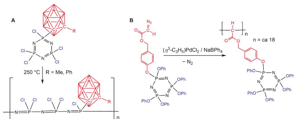
**Scheme 3.** Examples of polymerization reaction of AB<sub>5</sub> derivatives of cyclotriphosphazene. (A) Polymerization of N<sub>3</sub>P<sub>3</sub>. (B) Polymerization of a substituent of N<sub>3</sub>P<sub>3</sub>.
