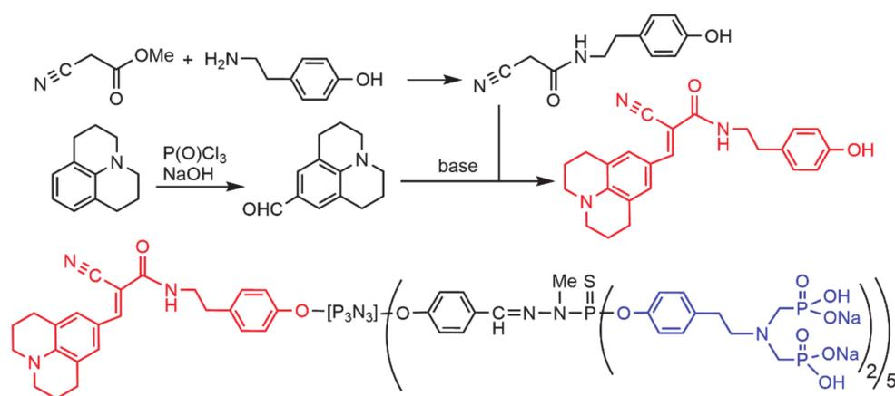
**Figure 8.** Synthesis of a julolidine derivative, and its use for the functionalization of an azabisphosphonate dendron.
