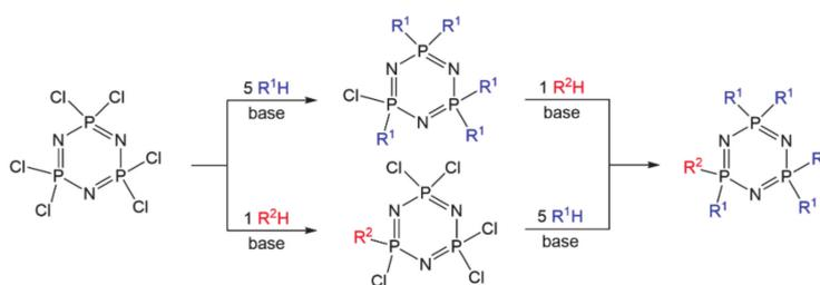
**Scheme 1.** Two ways for the synthesis of AB<sub>5</sub> derivatives of cyclotriphosphazene.
