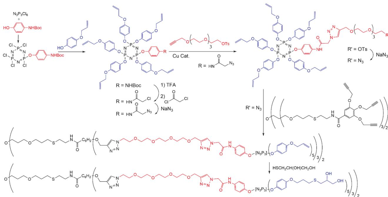
**Scheme 5.** “Onion peel” (layered) dendrimers having one layer of cyclotriphosphazenes ( $\text{N}_3\text{P}_3$ ), and synthesized via click reactions between alkynes and azides.
