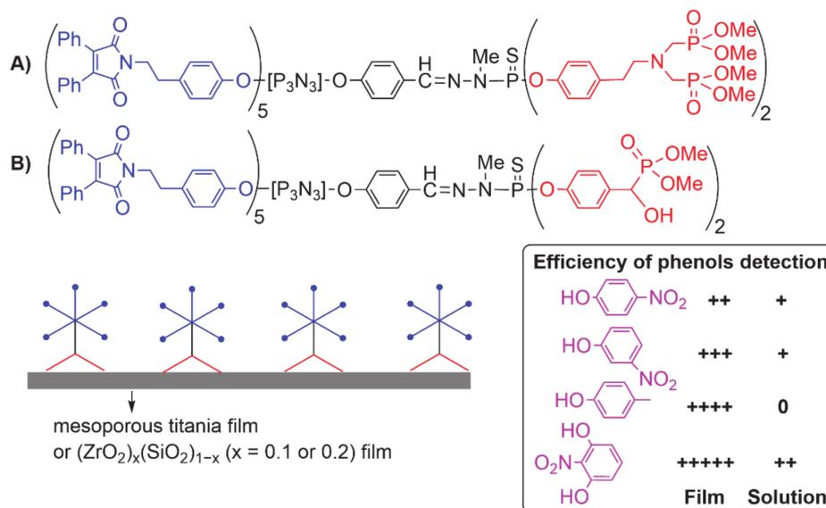
**Figure 2.** Dendrons grafted to solid surfaces. (A) Dendron grafted to mesoporous titania films. (B) Dendron grafted to  $(ZrO_2)_x(SiO_2)_{1-x}$  films surface. In the frame: efficiency of the dendron shown in (A) on titania or in solution for the detection of nitrophenols.
