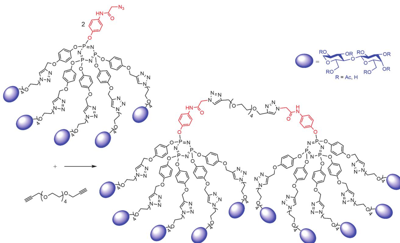
**Scheme 8.** Dumbbell-shape dendrimer obtained by a double “click” reaction onto dipropargylated tetraethylene glycol.
