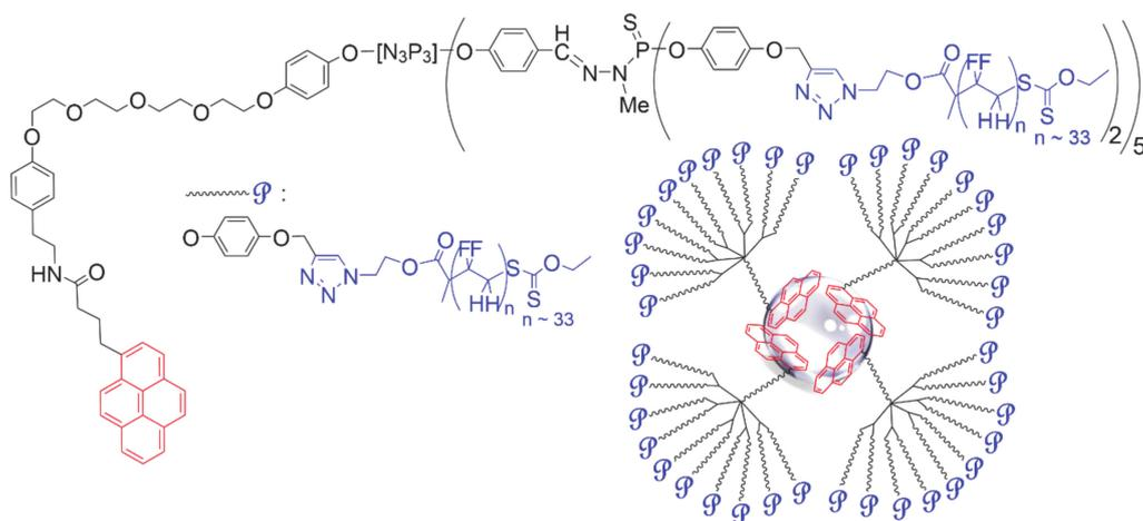
**Figure 4.** Chemical structure of a dendron bearing vinylidene fluoride polymers on the surface, and used for coating cobalt nanoparticles covered by graphene.
