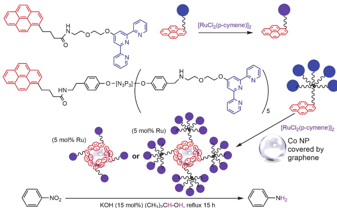
**Scheme 13.** Another example of non-covalent grafting of catalytic dendrons onto cobalt nanoparticles covered by graphene layers. The lower part of the Scheme displays the catalyzed nitroarene transfer hydrogenation from 2-propanol.
