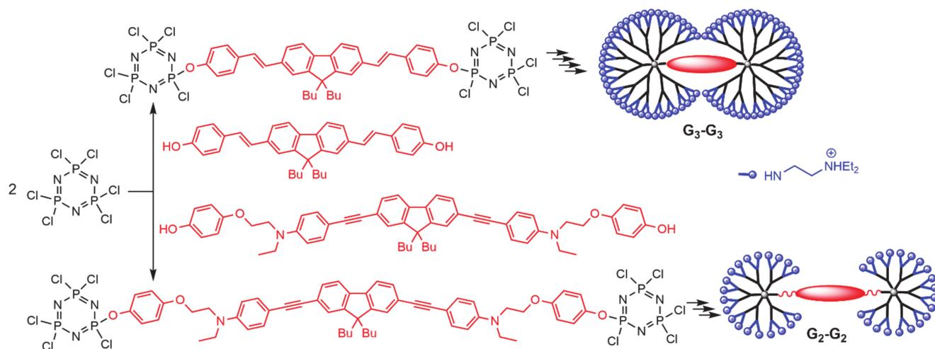
**Scheme 7.** Synthesis of “dumbbell-shape” dendrimers having two  $AB_5$  derivatives of  $N_3P_3$  linked to a fluorescent core.
