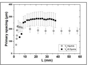
Figure 3: Primary spacing evolution as a function of the solidified length L for  $V_P = 4 \mu m/s$  and  $V_P = 0.5 \mu m/s$  (G = 19 K/cm).
