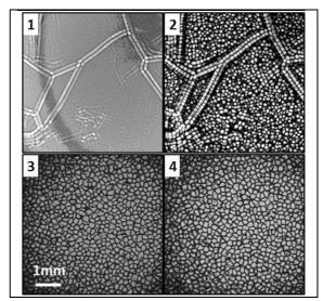
**Figure 2:** Development of morphological instability initiating on subboundaries. Once the pattern is well developed, subboundaries are no longer visible.  $t_1$  = 1.6h,  $t_2$  = 1.8h,  $t_3$  = 2.7h,  $t_4$  = 4h ( $V_P$  = 1  $\mu$ m/s; G = 19 K/cm)
