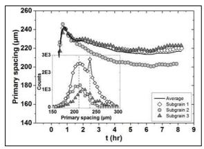
**Figure 5:** Primary spacing evolution: average on the whole interface, and by subgrain. The histograms correspond to the distributions by subgrain at t = 5.5h, integrated on successive images on a duration of 0.4 h ( $V_P = 2 \mu m/s$ ; G = 19 K/cm).
