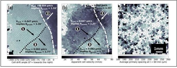
Figure 4: Analysis of the drifting velocity of cells to identify subgrains: drifting direction in a) and drifting velocity in b). 3 subgrains are identified; their average drifting velocity, direction and corresponding misorientation of the <100> direction with respect to the thermal/optical axis are given. c) Mapping of primary spacing of cells at t = 1h. ( $V_P = 2 \mu m/s$ ; G = 19 K/cm).
